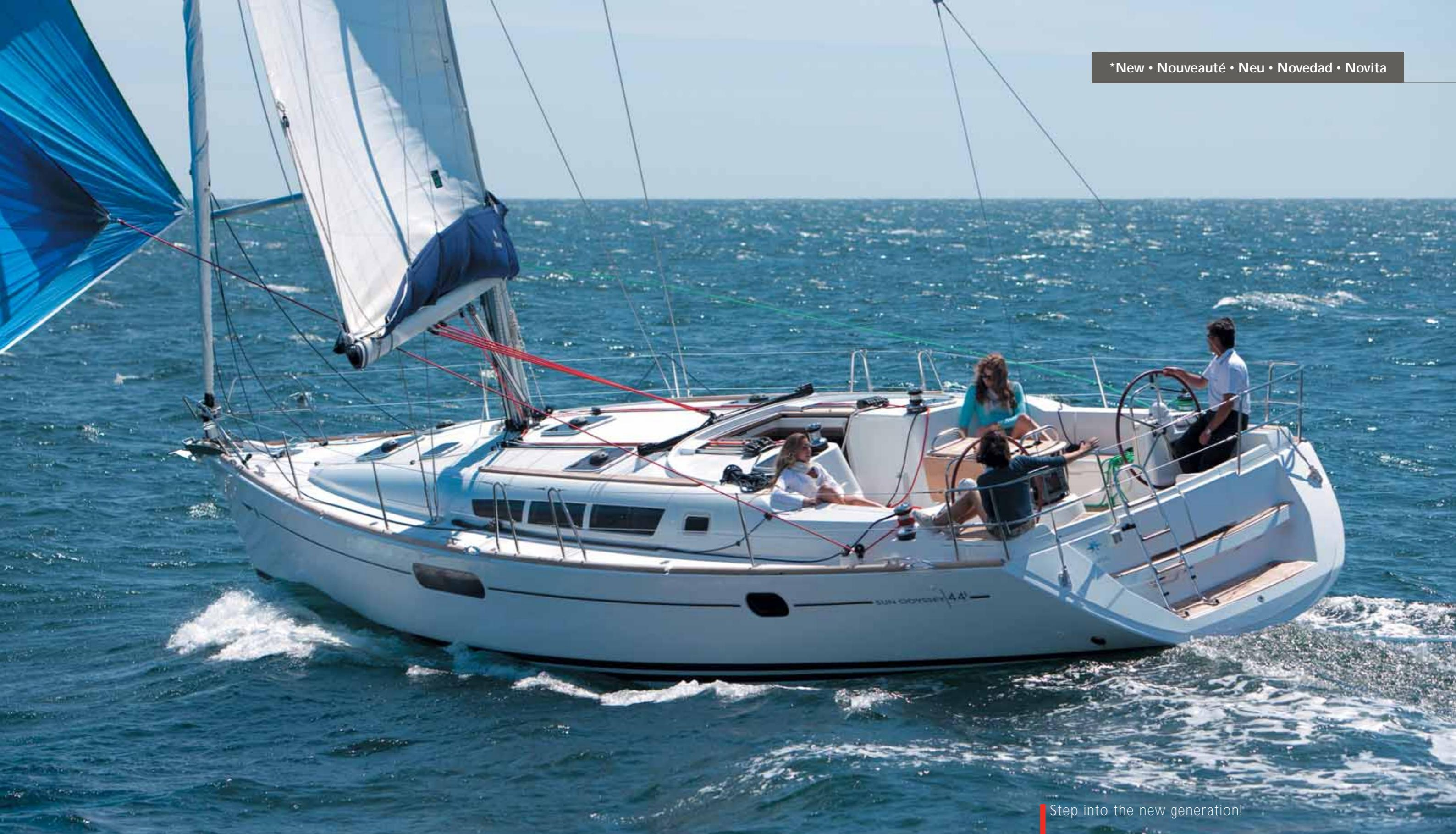
The Performance version of the Sun Odyssey 44i is designed for even more power and speed, fitted with Prestige series sails, tri-radial cut in Mylar/Taffeta, a taller mast, twin groove furler, a feathering propeller and more, allowing you to go faster while enjoying the same comfort offered on the standard version.
